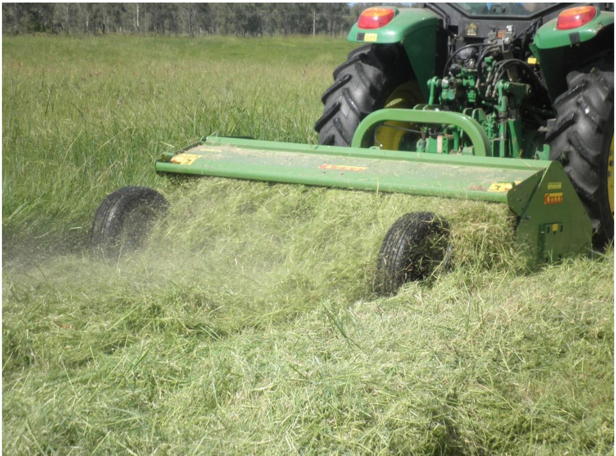
1. **Oil:** All machines need oil and mulchers are no exception. The gearbox oil should be changed each year. They hold only a small amount of oil, normally gear oil (check manufactures recommended oil) and contaminants build up and reduce the lubrication efficiency of the oil and ultimately more expensive gearbox failure. Most gear boxes will have a drain plug, a filler plug and a breather. Be sure to fill to the correct level as indicated in the operator's manual.
